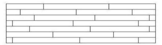
11. Continue installing the remaining rows following the same instructions above and keeping note of all the requirements. Once all the flooring is laid you can go over the floor with a heavy roller to ensure the plank has bonded to the adhesive successfully (optional). Install the removed molding/ skirting or if you have undercut the jambs or laid the planks up against the molding/skirting you can cork/silicone/gap fill the gaps around the parameter for a clean finish.
