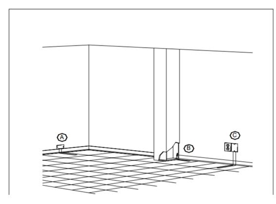
Common accepted ESD Tile system grounding methods
